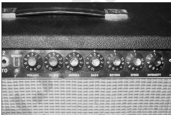
Figure 2-9: Place the controls in a neutral position with the volume reduced, effects off, and tone controls “flat.”
