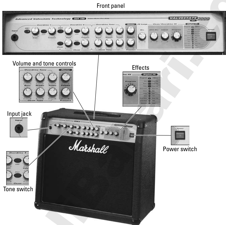
Figure 1-2: A typical guitar amp with its major parts labeled.
